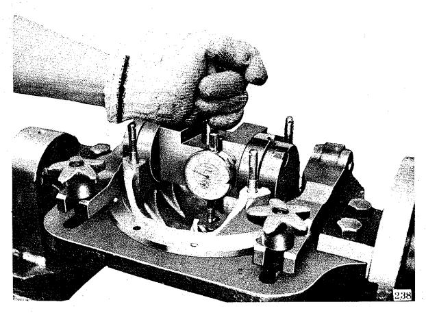
Fig. 9 Adjustment of Pinion Height
