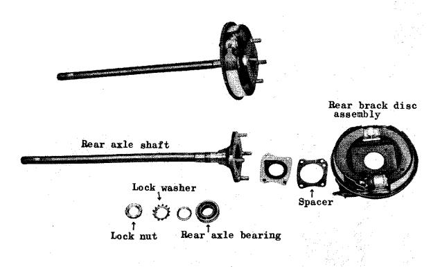
Fig. 2 Rear axle shaft & brake disc assembly
