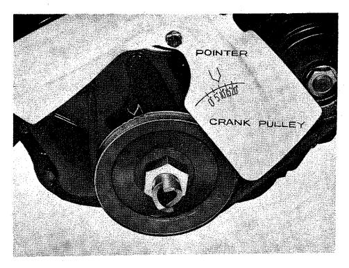
Fig. 1 Checking the Ignition timing
