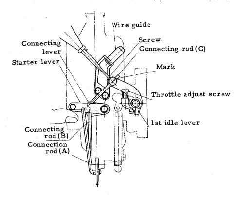
Fig. 6 Adjustment for Openning degree at connecting
