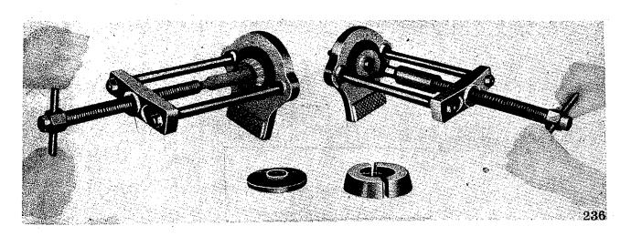
Fig. 5 Inner race replacer
