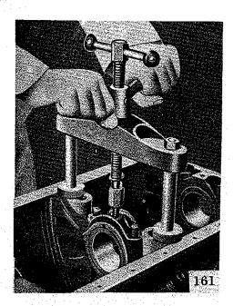
Fig. 14 Removing a Main Bearing Cap & Extractor
