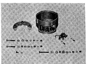
holder (23133-12210) from the rear cover, when be careful not to lose small parts such as screws, washers and bushings.
