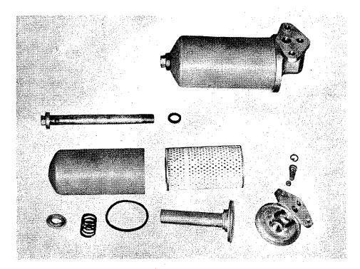
Fig. 3 Component of oil filter
