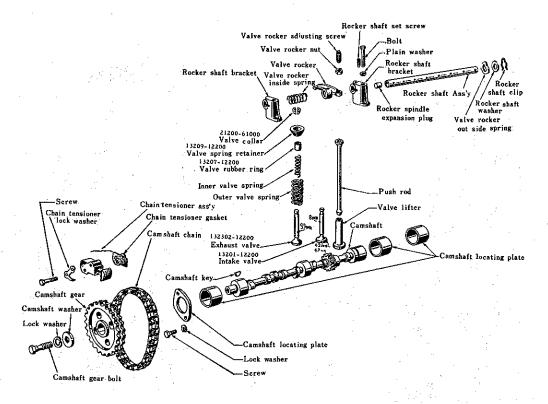
Fig. 10 Cameshaft & valve gear
