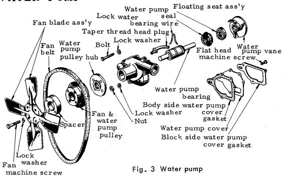
After draining the water from the radiator, remove the pump unit from the cylinder block by taking off the fan belt and releasing the setbolts with spring washers and hinge bolts to dynamo.
