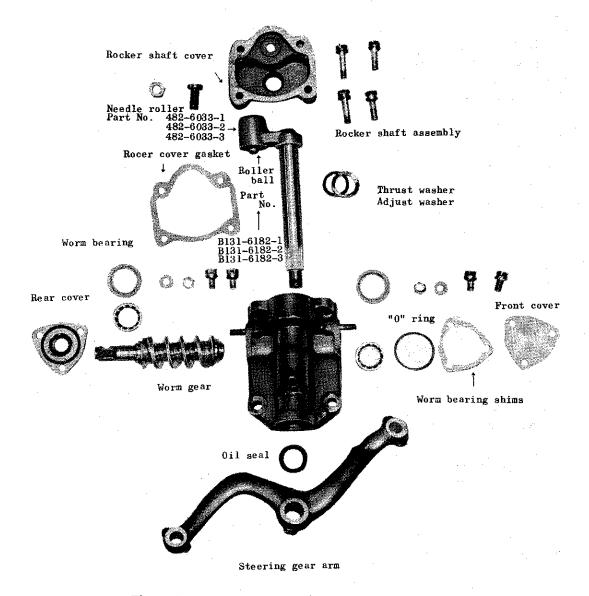
Fig. 5 Components of the steering gear case
