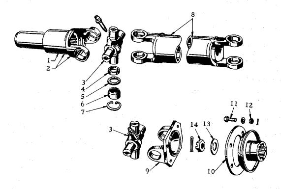
Fig. 1 Propeller shaft & joint
