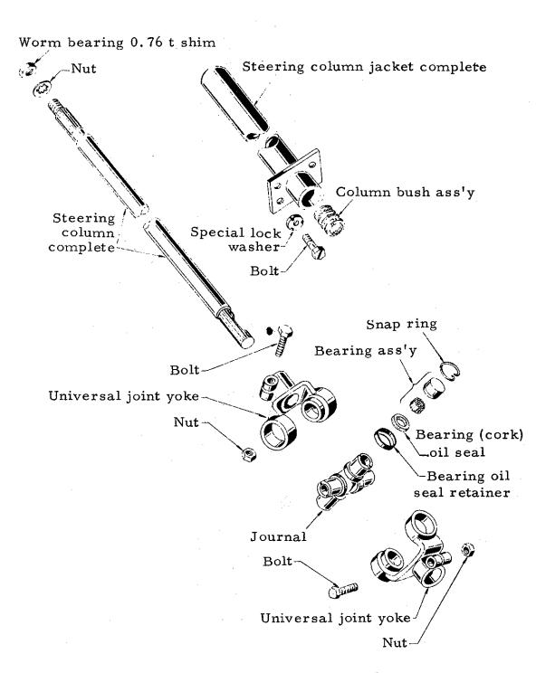
Fig. 4 Steering column & coupling
