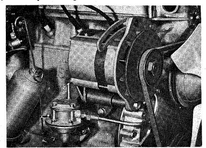
Fig. 2 Fan belt adjustment
