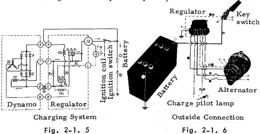
When the ignition switch is put on, the battery current flows in the arrow marked direction passing through the dynamo E terminal, brush slip ring, field coil, slip ring, brush, dynamo F terminal, relay F terminal and IG terminal and completes the field circuit. It in difficult for the dynamo to stand up only by residual magnetism of the field core, so that magnetization is necessary until voltage rises to suit charging after the engine has started.
