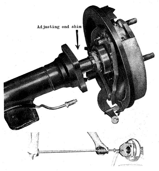
Fig. 1 Removal of axle shaft and disc assembly
