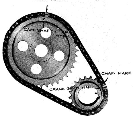
Fig. 2 Position of refitting gears with the chain
