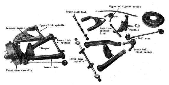
Fig. 4 Front suspension member
