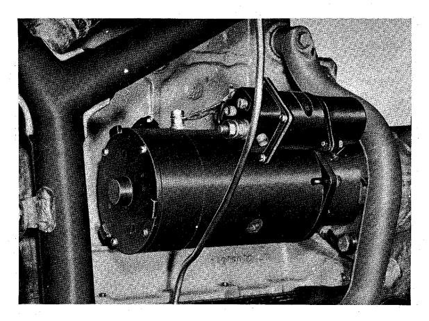
After the engine starts and its speed becomes greater than the no-load speed of the starter, the pinion is kicked back to unmesh and return to its former position.
