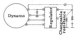
Connect the battery almost charged in full as shown, and make the dynamo revolution with 4000 rpm.
