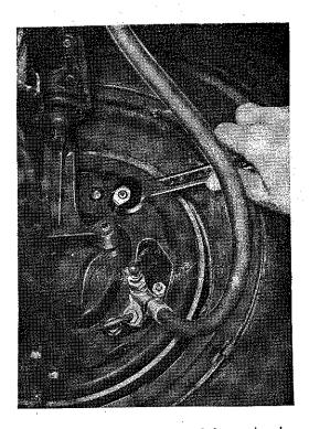
Fig. 2 Adjusting of front brake
