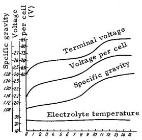
Fig. 3 Constant current charging characteristics
