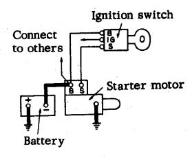
Fig. 5 Magnetic Starter Circuit
