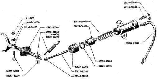
Fig. 2 Clutch operating
