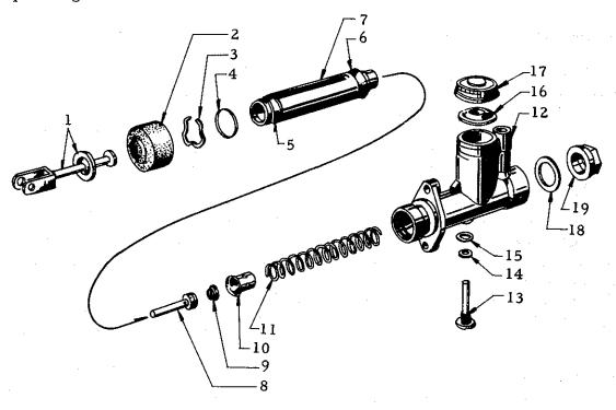
Fig. 1 Components of the master cylinder
