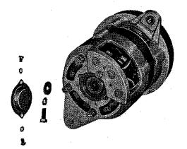
Remove the cover (23130-12210) of bearing (23129-12210, JIS #62022 ZZC3) and take off the hex. bolt of shaft.
