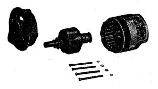
Remove the throu bolt (23131-12210) tightening bolt front cover (23118-12210) and rear cover (23127-12211), pull off the front cover and rotor (23108-12210). Use a hammer of wood or plastic if necessary.
