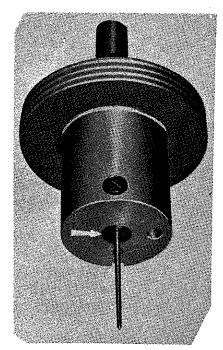
Fig. 10 Setting Jet Needle
