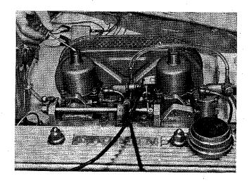
Fig. 7 Inspecting Damper Oil
