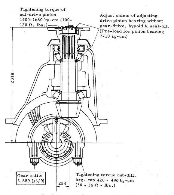
Fig. 3 Section of differential case
