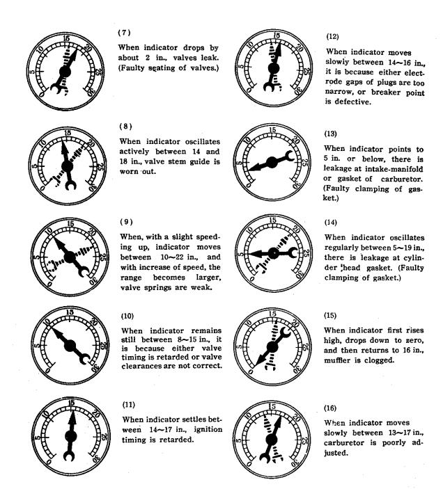
Fig. 3 Diagnosing engine by means of a vacuum gauge
