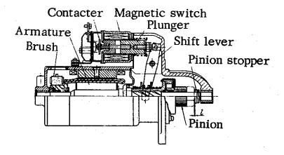
Fig. 1 Sectional view of magnetic shift type
