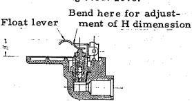
Fig. 5 Adjusting Float Level
