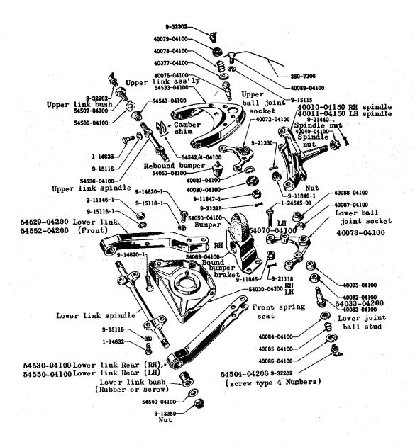
Fig. 2 Front suspension
