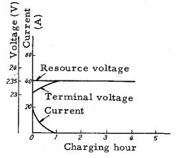
Fig. 4 Constant voltage charging characteristics
