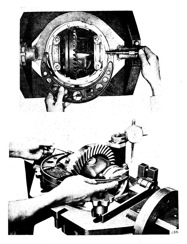
Fig. 17 Using the differential side bearing cap gauge
