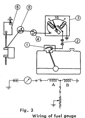
If not normal, remove tank unit and adjust the bend of the pipe.
