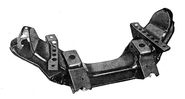
Fig. 2 Front suspension member
