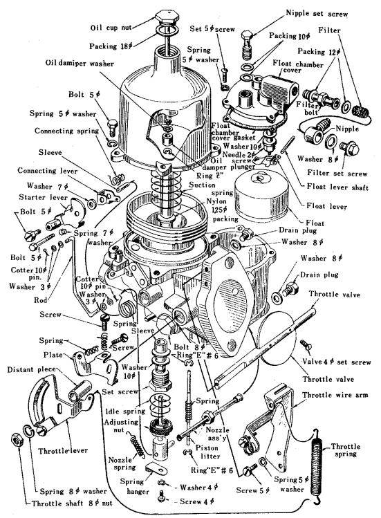
Fig.9 Key to the Carburetor Components
