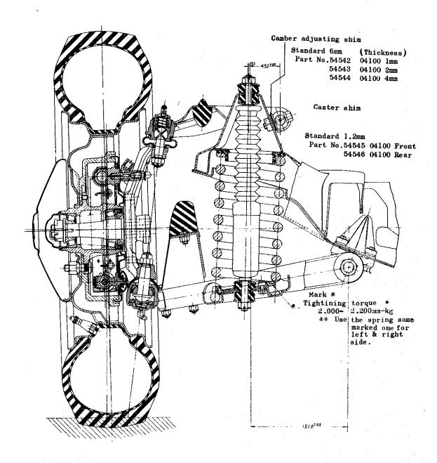
Fig. 3 Section of front suspension
