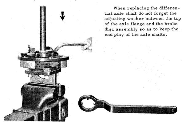
DT-4680 Rear axle shaft bearing lock wrench
