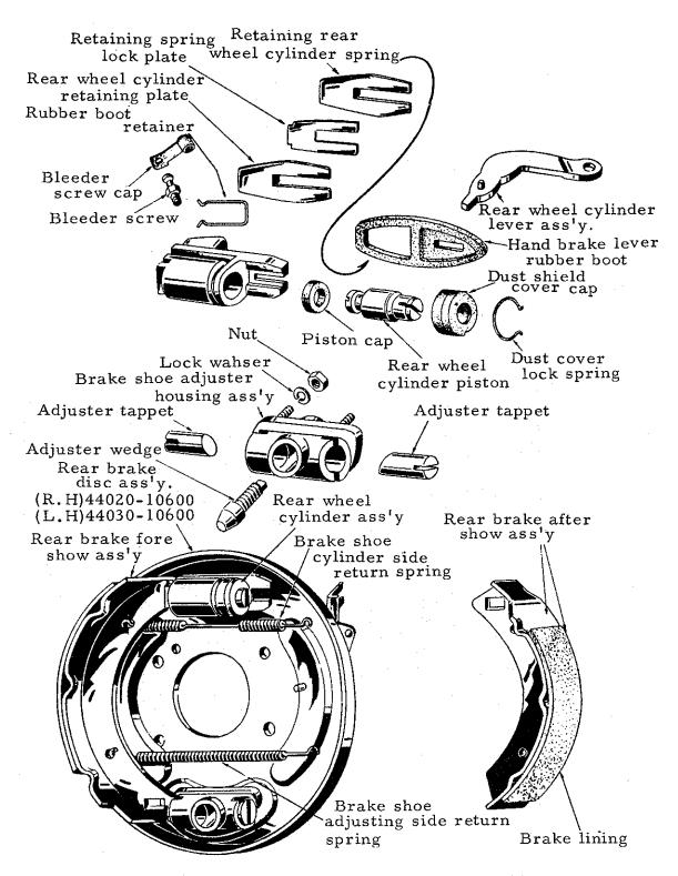
Fig. 4 Components of rear brake
