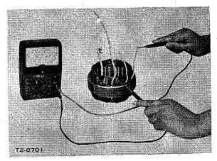
If the terminal connected to the diode is not conductive with the stator core, that is all right.
