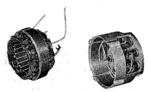
Remove the rear cover and stator (23102-12210). Separate the silicon diode, 3ea. from the stator coil lead wire, 3ea. by melting soldering with an electric iron. Slacken N terminal bolt on the rear cover side and remove the clip terminal, then the rear cover and the stator can be separated.
