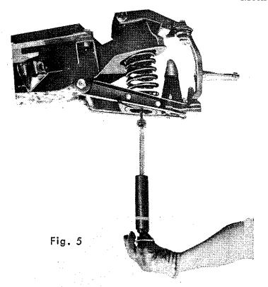
Method 1 Lift the side or front bumper of the car concerned and place blocks under the body unscrew nut of the shock absorber at the top and take out it from down side after unscrew lower small flange of it from lower spring plate.
