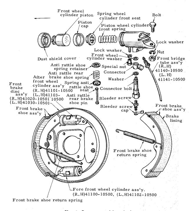
Fig. 1 Component of front brake
