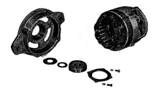
Remove the ball bearing From Front cover. Remove the bolt or (23352-09610) tightening the ebearing plate (23123-12210) and tor pull off the bearing with such as a hand press.
