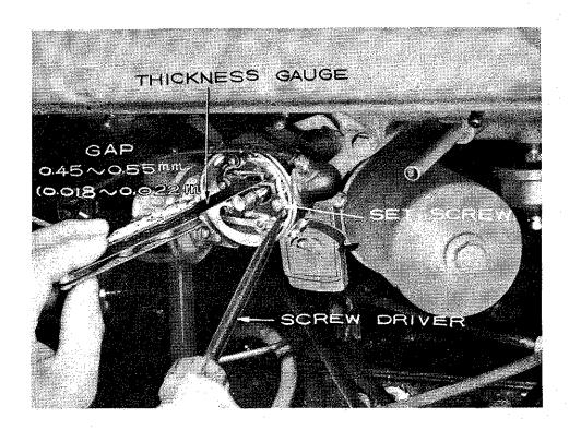
Fig. 15 Adjusting the Point Gap
