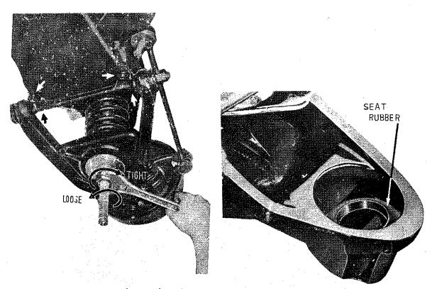
Fig. 7 Refitting the coil spring
