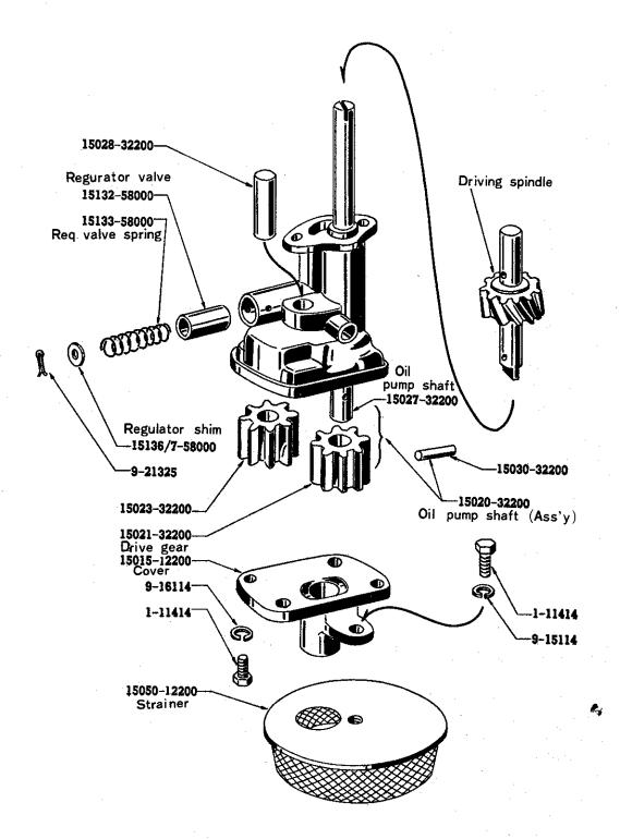
Fig. 6 Oil pump & strainer assembly
