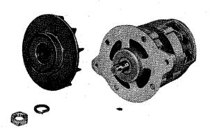
Remove the hex. nut (23153-12210) of pulley (23151-12210) and pull off the pulley and the half-moon key (23195-12210). Be careful not to injure the fan when the nut is removed.
