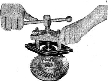
Fig. 1 Using of side bearing puller (DT4686)
