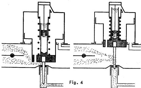
Full open low speed operation. Full open high speed operation
